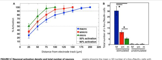
activated. (A) Mean  $\pm$  SD percentage of neuronal activation% in 25  $\mu$ m radius increments surrounding implanted and stimulated electrodes. (B) Bar
