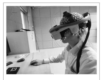
FIGURE 7 | Electroencephalogram recording in 3DI virtual reality environment.
